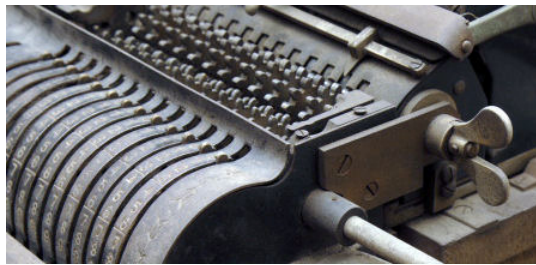
Figure 6.2 - Thompson's difference engine, the transfer mechanism
